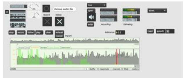
Figure 8: The green signal represents a new gesture that is probabilistically compared to the already recorded grey signal, allowing for the following of the performance by the system according to a threshold of tolerance
